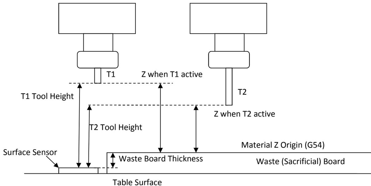
Each tool that is to be used in a job must have a tool height so that the machine can figure out where it is relative to the Material Z Origin (G54) (surface of the waste or sacrificial board).
